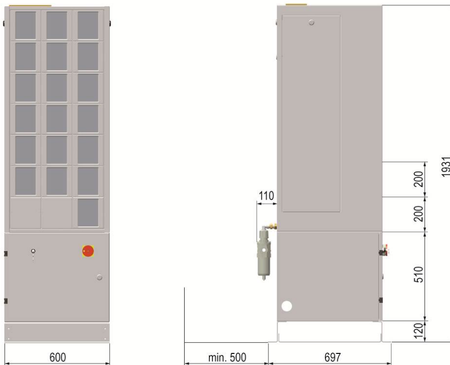
OptiFlex A2 Control system - set-up
